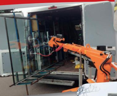
The Smartlift can be shifted sideways for precision adjustment during installation jobs.
