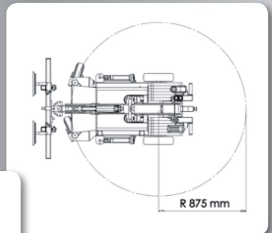
*The two powerful 1500 W electric motors mean that the SL 208 Compact can rotate on its own axis. All it requires is a firm surface.*
