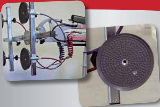
The SL 208 Compact comes as standard with lifting yoke, suction cups and dual circuit vacuum system for handling windows etc.
