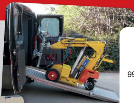
The SL 380 Midi can be shifted sideways up to 3.9 in for precision adjustment during the window installation process.
