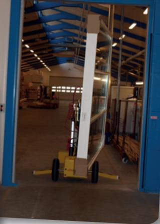
The SL 580 Maxi can be shifted sideways up to 3.9 in for precision adjustment during the window installation process.
