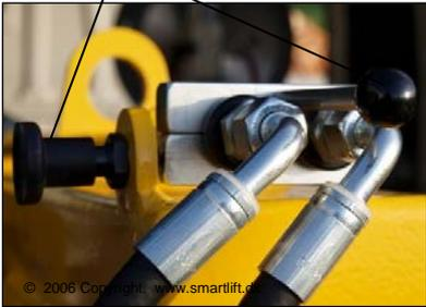
11 – Hose couplings for 2 circuits BLUE CIRCUIT / RED CIRCUIT
