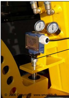
The telescopic arm is run back in, and work too heavy for the machine is lowered back in place. Should the safety switch switch off again at this manoeuvre, you may, using your body weight, push the machine in place by applying pressure on the weight blocks. Possibly release safety switch using a screwdriver.
