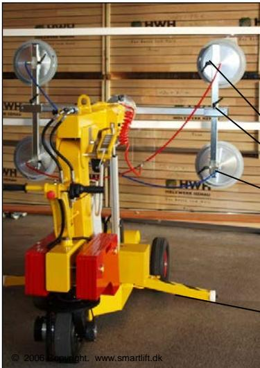
For max. stability at transport of sucked work, the suction cups are to be centred and adapted to the transport work chosen. ***Operation of yoke with sucked work should always be conducted with caution***
