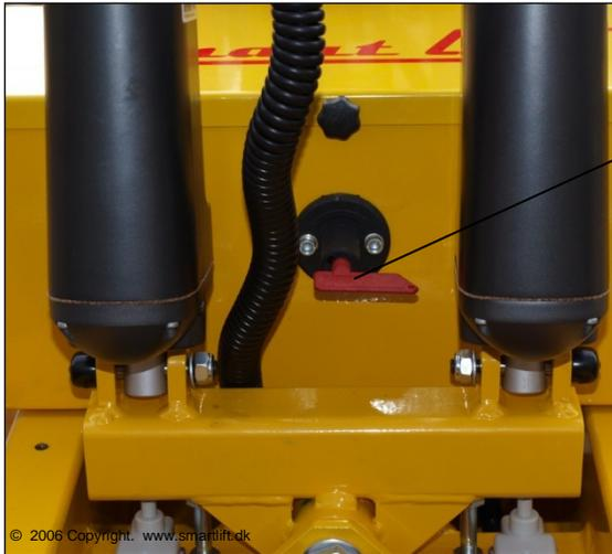
38 – Main Switch, switching off all functions on el. on the machine
