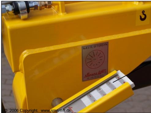
32 – Operation panel placed in special holder on the machine right hand side. May be kept manually free out of holder but be aware that the connector may not come loose at the control box
