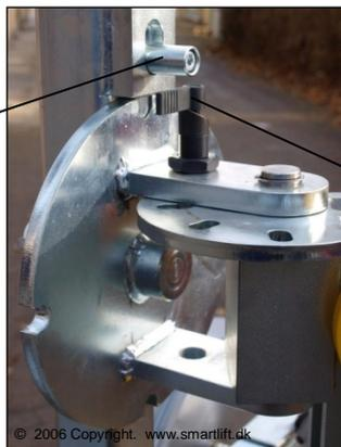
Positioning bolt. Keeping the turning head locked in fixed position when yoke is required to be turned to one of the sides. Span 180°
